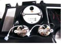
Connect the black ground wires from the lamp pigtails to the center ground studs of the smaller gauges as shown.
