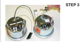
Install appropriate lamp socket pigtails into the speedometer & tachometer.
