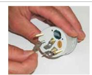
Install the blade terminals to the back of each of the 4 small gauges. Secure with lock washer and nut. There are specific left, center, and right hand terminals. Install as shown in photo
