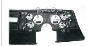
Install the mounting brackets on all the 6 gauges. The completed assembly is now ready for the connection of the wiring harness. Note that this assembly shows Series I gauges.
